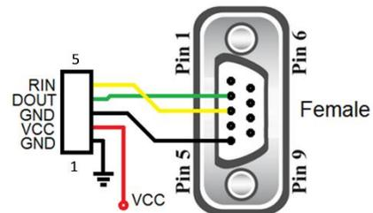
Figure 6: Electrical Schematic of RS-232 Cable: 10-CARS-EXT)
