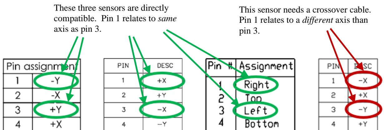
Figure 21: Connector Pinout Tables for Example 4-Wire Resistive Touch Sensors
