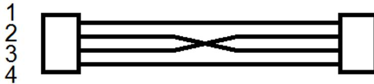
*Figure 22: Electrical Schematic of 4-Wire Crossover Cable*
