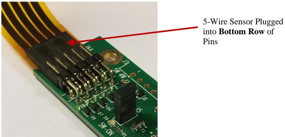
*Figure 2 : Properly Connected 5-Wire Resistive Touch Sensor*
