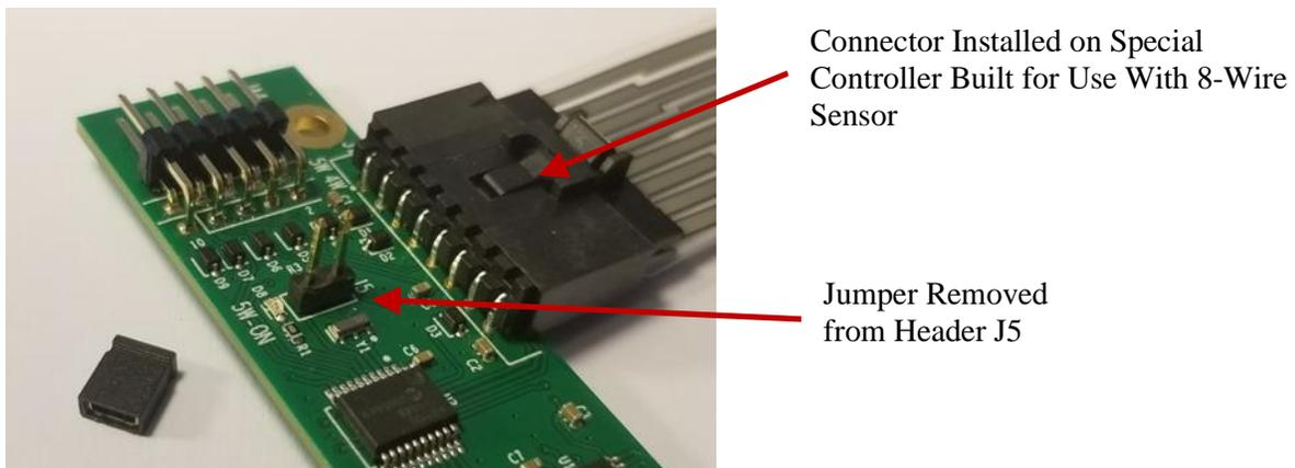
Figure 26: Remove Jumper from Header J5 to Use an 8-Wire Sensor
