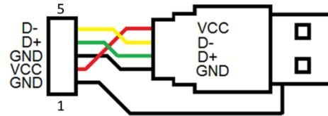
Figure 4: Electrical Schematic of USB Cable: 10-CARU-EXT)
