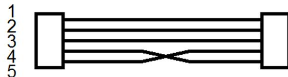
Figure 20: Electrical Schematic of 5-Wire Crossover Cable
