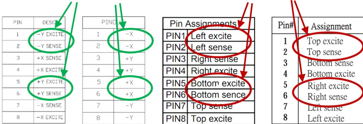
Figure 27: Connector Pinout Tables for Four Example 8-Wire Resistive Touch Sensors
