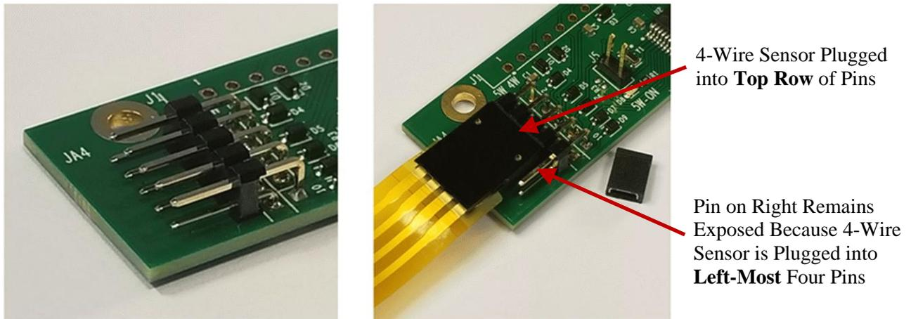
*Figure 3: Use the Left-Most Pins of Header JA4 Top Row to Connect 4-Wire Sensor Flex Tail Connector*
