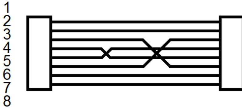
*Figure 28: Electrical Schematic of 8-Wire Crossover Cable*
