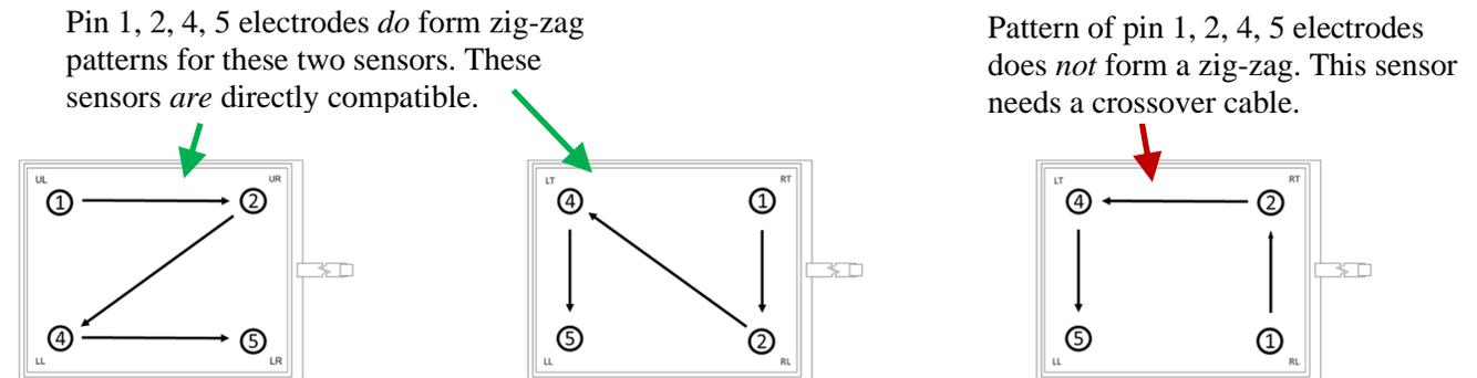
Figure 19: Pinout Patterns of Example 5-Wire Resistive Touch Sensors
